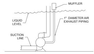
Pump can be submerged if the pump materials of construction are compatible with the liquid being pumped. The air exhaust must be piped above the liquid level. When the pumped product source is at a higher level than the pump (flooded suction condition), pipe the exhaust higher than the product source to prevent siphoning spills.
